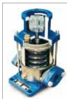
**2. The electric pilot pump,** vertical with wetted parts in AISI 304 stainless steel, guarantees utmost resistance to corrosion durability, easy and fast maintenance operations.
