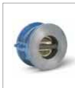
**4. Dual head non-return valves,** made of GG 25 cast iron with bronze elements and rubber sealing ring, they have extremely reduced overall dimensions and weights, and considerable working advantages: wide passing section for very low pressure drops, water hammer dampening, facilitated inspection and easy maintenance.
