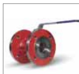
**3. The full bore flanged ball valves,** made of GG 25 cast iron with brass ball, teflon seal and low operating strain lever. Their smooth rubber and high quality materials guarantee best sealing properties even after many years.
