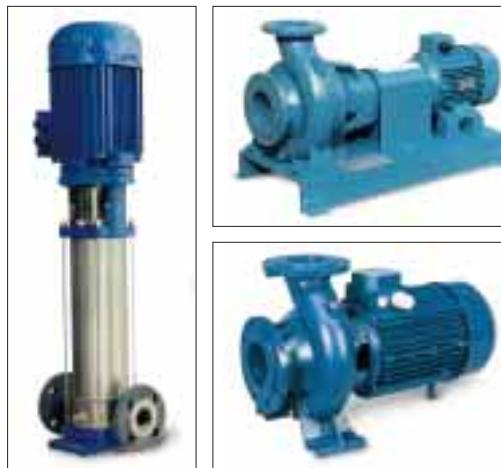
**1. The main pumps** either horizontal single-stage or vertical multistage. Easy and quick disassembly of all rotary parts is performed from the motor side without disconnecting the intake or the delivery pipes.
